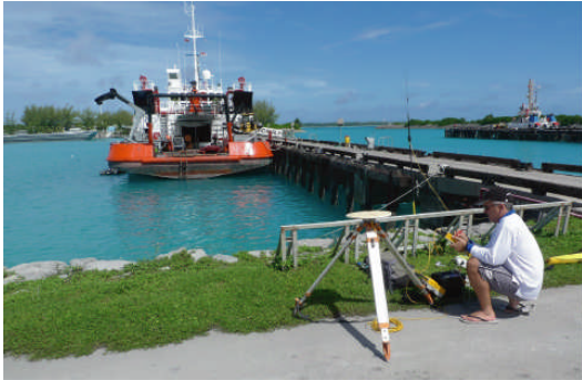
Fig. 3 Scott operating our RTK receiver on Diego Garcia with the Pacific Marlin in the background. This device gives precise elevation and spatial data using satellites. Photo Sarah Woodroffe
